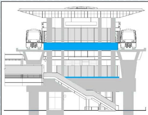
**3 Concrete is placed for the circulation level and platform.** Once the concrete slabs reach the prescribed strength, they are polished to create the station's finished floor.
