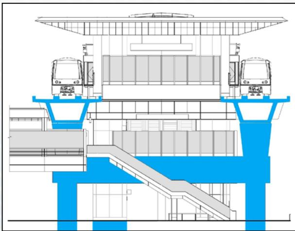
**1 The guideway is constructed.** Concrete is placed for underground foundation elements (cast-in-drilled-hole piles and elevator pits) and the above-ground guideway structure.
