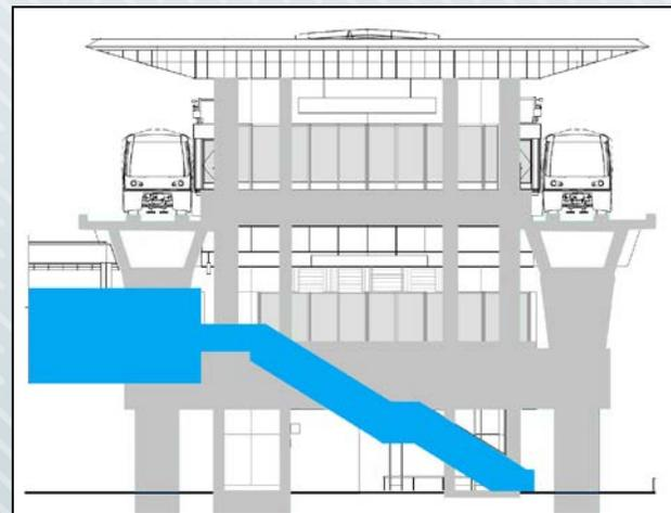
**4 Station access facilities are constructed.** The stairs and pedestrian walkways provide access to the station and connect to parking facilities and the airport terminals.
