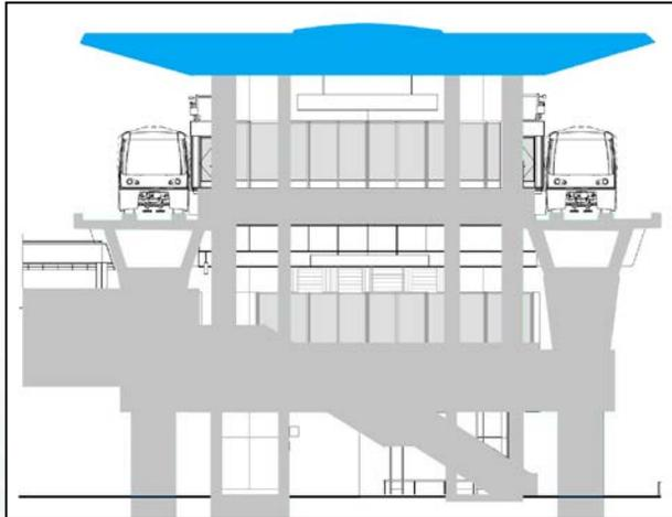
**5 Station canopy is erected.** The station's canopy, which includes its 20-foot diameter circular skylights that will help illuminate the platform, is built.
