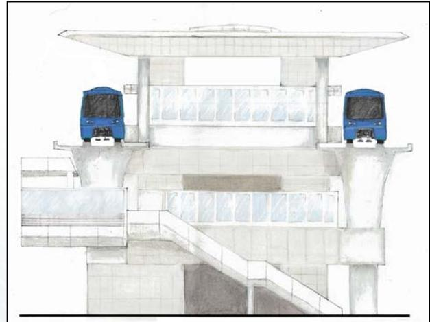
**6 Elevators, escalators, utilities and architectural finishes are installed.** The station's final elements are completed to prepare the station to open to the public.
