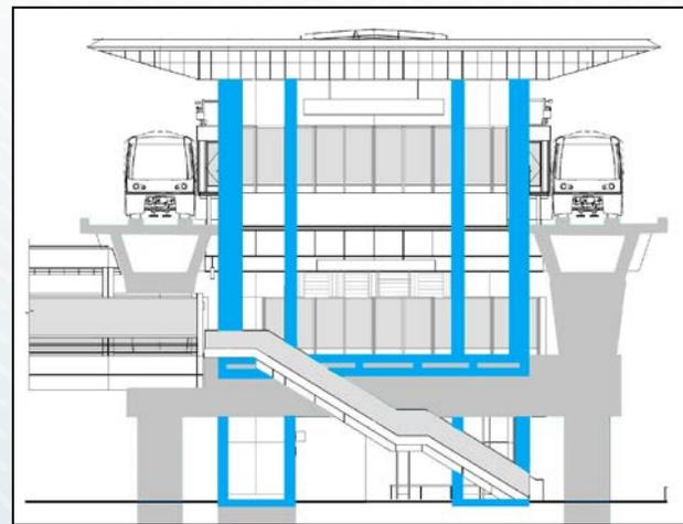
**2 Station steel is erected.** The station's shell and elevator shafts are established to support constructing the elevated station.
