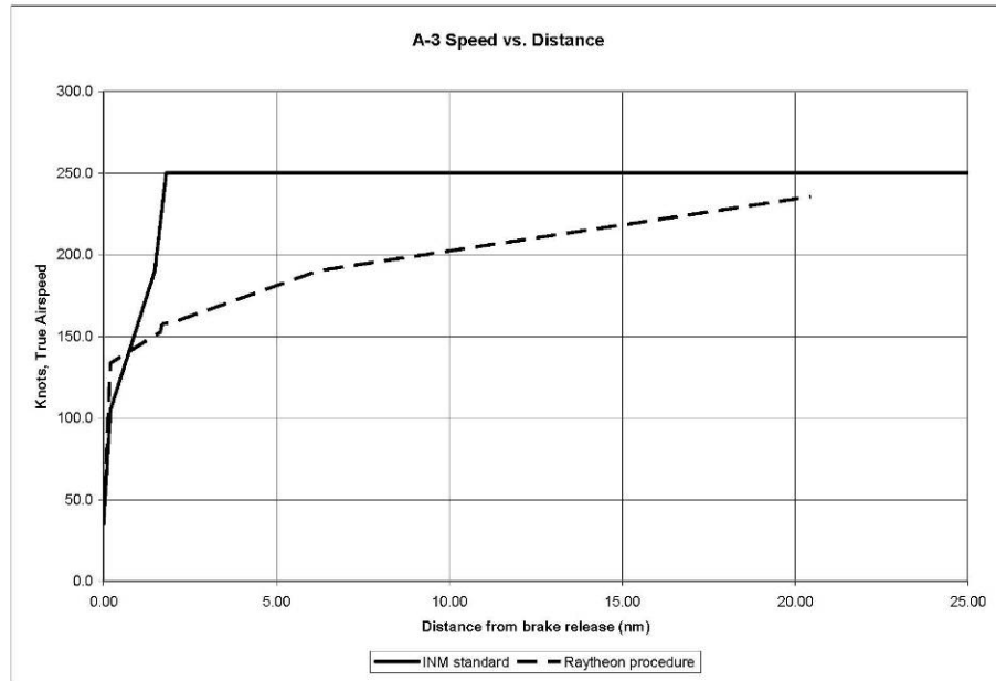
Figure 2. Airspeed Profiles for Standard and Raytheon Procedures
